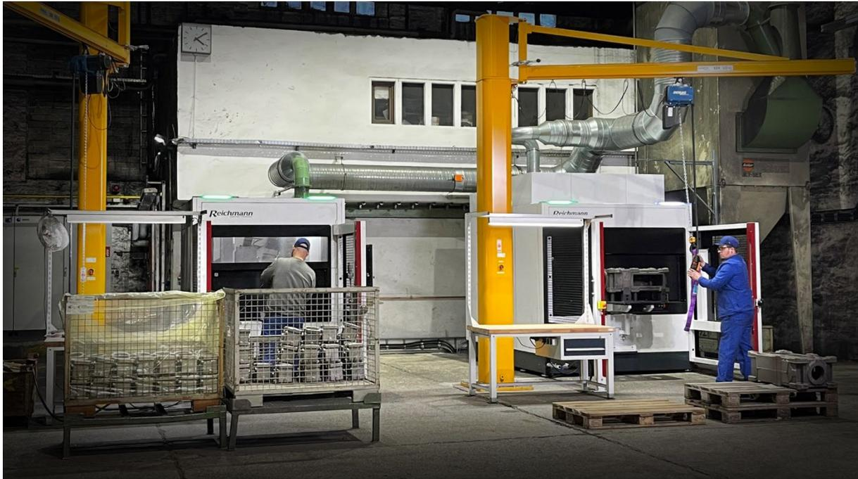
**High time savings, staff relief and an improved, reproducible grinding quality: The German foundry Schmiedeberger Gießerei already benefits from all these advantages with the first automatic grinding machine from Reichmann – and would like more of it. The combination of the Maus 600 with the new Maus 900 expands automatic casting finishing for the foundry's wide range of castings.**
